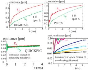
Figure 5: Results of instability simulations for the example case by various codes: HEADTAIL with 1 IP (top left), PEHTS (top right), QUICKPIC (bottom left), and HEADTAIL with various numbers of IPs for both open and conducting boundaries .
