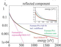
Figure 2: Different parametrizations of elastic reflection: formula (6) [5] [red], expression (5) [green], alternative (7) with  $\delta_{\rm el0} \approx 0.5$  [purple], and parametrization (9) which approximates [9], and includes a rediffused component [blue]. The inset shows a detail of the plot at low energy on a normal non-logarithmic scale.
