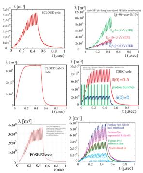
Figure 1: Results of build-up simulations for the example case by various codes: ECLOUD with (3) (top left), EPI and PEI (top right), CLOUDLAND (centre left), CSEC (centre right), POSINST (bottom left), ECLOUD using the four parametrizations of Fig. 2 [same colors] and a fifth case without elastic reflection [cyan] (bottom right).
