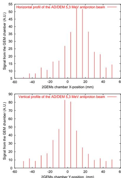
Figure 3: Profiles from a double GEM monitor on the AD beam line.
