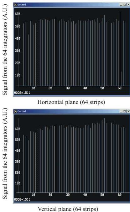
Figure 2: Gain uniformity of the triple GEM monitor with a 70/30 ArCO<sub>2</sub> gas mixture. Irradiated by 90<sup>Sr</sup>.
