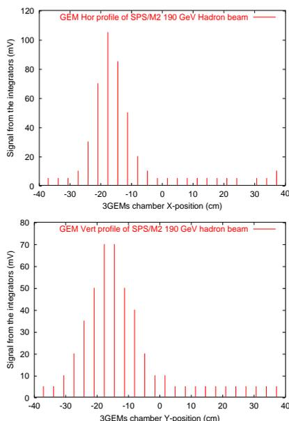
Figure 4: Profiles from a triple GEM monitor on the SPS/M2 beam line.
