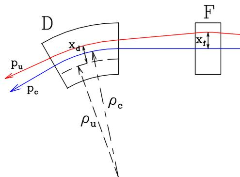
Figure 1: Layout of FODO cell with D-sector and F-quad.
