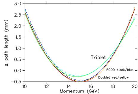
Figure 5: Pathlength variation in muon lattices F2,D2,T2
