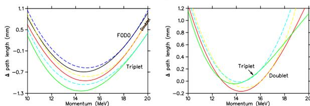
Figure 9: Pathlength variation in electron lattices F1,D1,T1 (left) and F2,D2,T2 (right).
