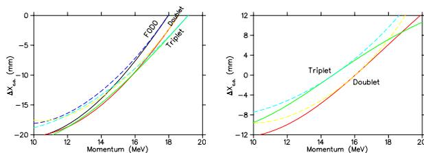
Figure 8: Closed orbit offsets in electron lattices F1,D1,T1 (left) and lattices F2,D2,T2 (right).
