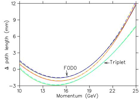
Figure 4: Pathlength variation in muon lattices F1,D1,T1
