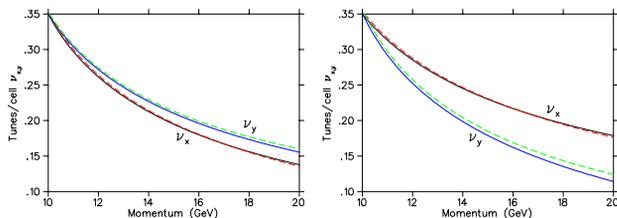
Figure 6: Tunes in muon lattices D2 (left) and T2 (right)
