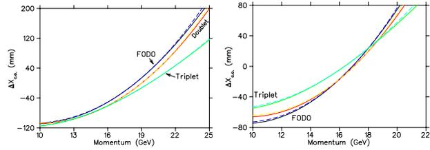
Figure 3: Orbit offsets in F-quad for lattices F1,D1,T1 (left), and in F-sector for lattices F2,D2,T2 (right)
