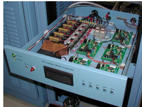
Figure 1: View of a chassis containing 5 shunt circuits
