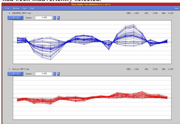
Figure 4: Horizontal (top) and vertical orbit modulation with a single shunt AC excited.
