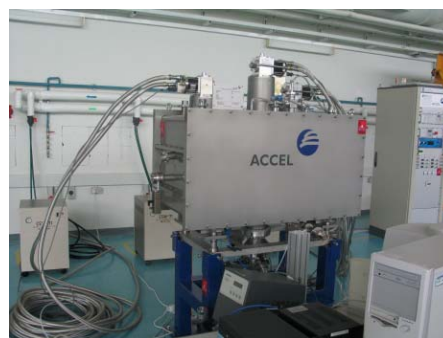
Fig. 6: Supramini (centre) during cool down at SLS. In the background, cryocoolers and power supply.
