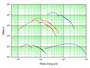
Fig. 2. Brilliance curves for the MAX IV rings. Blue curves: MAX IV X-ray ring Red curves: MAX IV soft X-ray ring Black curves: MAX II ring
