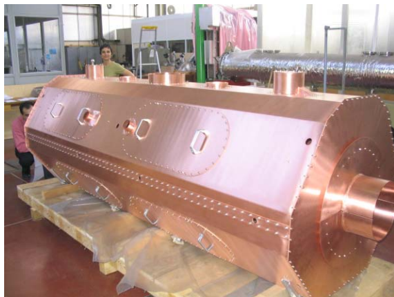
Figure 2: Copper thermal shield with 8 dismantable access doors.
