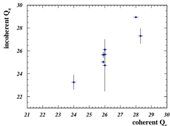
Figure 5: Incoherent synchrotron tune at a beam energy of about 2.5 GeV as a function of the coherent synchrotron tune. The incoherent tunes were determined from resonant depolarisation scans for different RF voltages, the coherent tunes were obtained from a beam frequency spectrum measured with a strip line.
