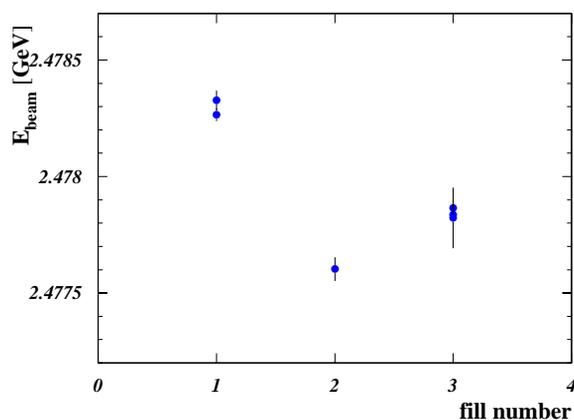
Figure 3: Results of the energy determinations at ANKA for different fills. It is clearly visible that reproducibility within fills is much better than between fills.
