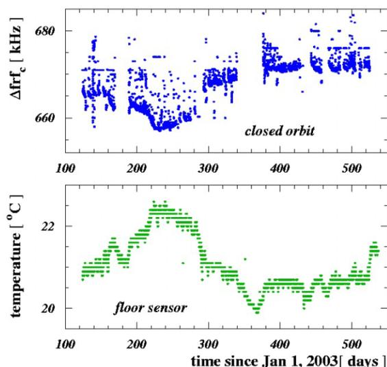
Figure 4: Upper plot: RF frequencies adjusted by the automatic closed orbit correction to match the central frequency as a function of time in days since January 2003. Lower plot: Temperature measured on the concrete floor of the ANKA building for the same period. The summer/winter differences are easily visible as is the anti-correlation between temperature and frequency.
