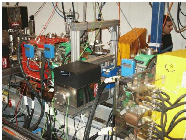
Figure 1: Picture of the Pb-Glass detector showing its location in the storage between two sextupoles (green), close to the maximum of the dispersion. The position of the detector is denoted by its aluminium frame mounting.
