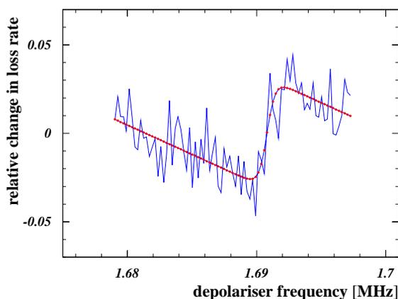
Figure 2: Relative change in loss monitor counting rate as a function of the depolariser frequency. The sudden jump in counting rate indicating the occurrence of a depolarisation is clearly visible. The measured rate is overlayed by the results of a fit (red points) according to Eq.(2).
