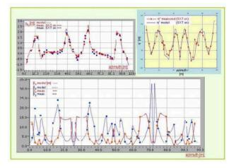
Figure 2: DA $\Phi$ NE model compared with beam measurements – up: first order and second order dispersion; down: beta functions.
