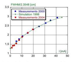
Figure 3: Bunch length measurements and theoretical predictions as a function of the bunch current for the positron ring.
