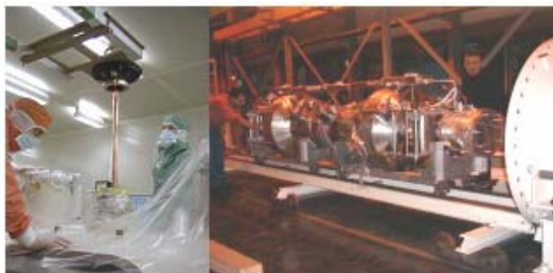
Figure 2: Cryomodule disassembling at CERN
