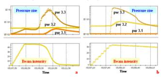
Figure 5: Evaluating NEG coating by observing pressure rise caused by beam loss, on the left, and by exciting electron cloud, on the right. The pressure rise at the gauge pw 3.2 is low in both cases, because of the NEG pipes. The location of pw 3.2 usually has the highest pressure rise.
