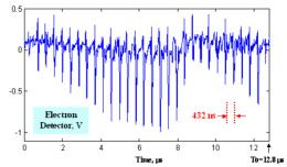
Figure 9: Electron multipacting of 28 bunches with  $1.7 \times 10^{11}$  protons per bunch, bunch spacing is 432 ns. Two beams with 10 ns bunch length meet at the location of the electron detector, with offset of 3 ns in time.
