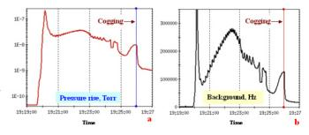
Figure 2: Transition pressure rise at high beam intensity caused experiment background problems. The pressure was reduced after beam cogging, but the corresponding singles rate was still 200 kHz, much higher than the coincident rate of 7 kHz.
