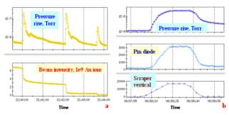
Figure 8: Left, gold beam collimation at 8.9 GeV/u. In all 3 incidents, ion desorption rates are  $\sim 1.5 \times 10^7$ . Right, vertical scraping caused pressure rise at 100 GeV/u. The deuteron ion desorption rate is larger than  $10^7$ .
