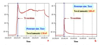
Figure 1: Typical transition pressure rise in the d-Au run. The left figure is with the total beam intensity of  $130 \times 10^9$  gold ions equivalent, and right figure is with  $100 \times 10^9$ . At the higher beam intensity, the high pressure lasted much longer.
