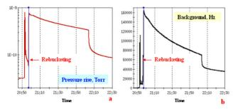
Figure 4: Rebucketing pressure rise and experiment background. Bunch length is shortened from 10 ns to 5 ns at rebucketing, which may have excited electron multipacting. The later sudden dramatic pressure reduction may be caused by the cease of multipacting.
