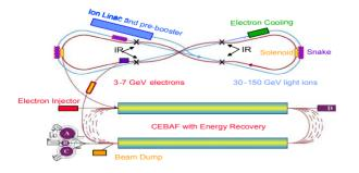
Figure 1: ELIC schematic lavout
