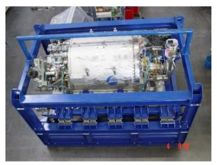
Figure 4: Completed SRF module for Cornell University installed into shipping frame.
