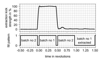
Figure 2: Normalized (100% = 0.6 mrad) measured kicker pulse and nominal fill pattern (2100 bunches per batch).
