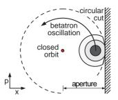
Figure 1: Phase space picture of beam loss at septum.
