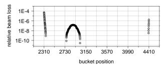
Figure 5: Relative beam loss, estimated from the initial betatron oscillation amplitudes after the extraction of the first batch.
