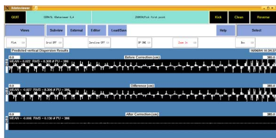
Figure 2: The dispersion correction of CLIC damping ring.
