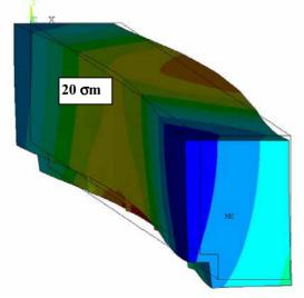
Figure 5: Deformation under thermal load of the 2-D C/C jaw in nominal conditions.
