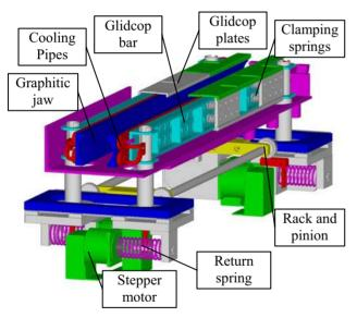
Figure 2: Horizontal secondary collimator components including motorization and actuation system.
