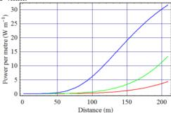
Figure 8: Power deposited along undulator length.
