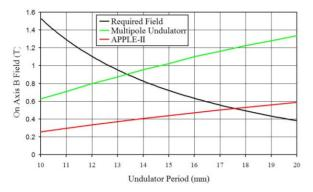
Figure 2: Required and calculated on-axis magnet field.
