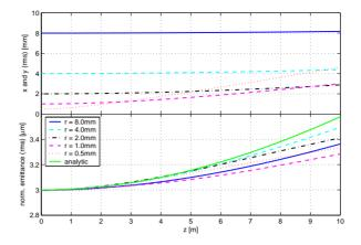
Figure 1: rms beam size and normalized emittance increase for  $\epsilon_0 = 3 \ \mu$ m, bunch length of 4 ps and charge of 80 pC.
