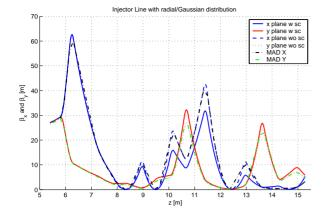
Figure 4:  $\beta$  function behaviour in the first (short) transfer line with and without space charge and original MAD matching.
