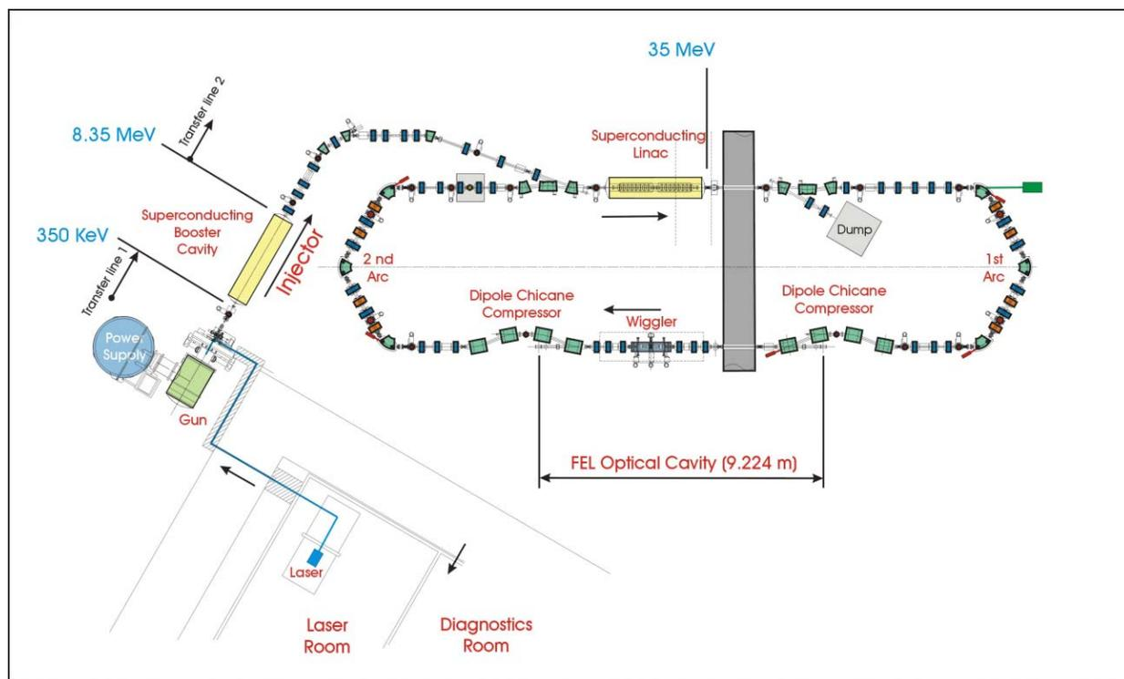
Figure 1: The layout of the ERL Prototype.
