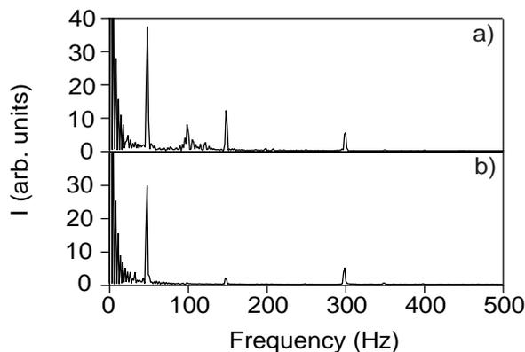
Figure 5: Power spectrum of the intensity signal  $I(t)$  for the ELETTRA FEL: (a) with derivative feedback only, and (b) with the derivative and proportional loops activated. (a) and (b) correspond to the signals of Figs. 3 and 4 respectively.
