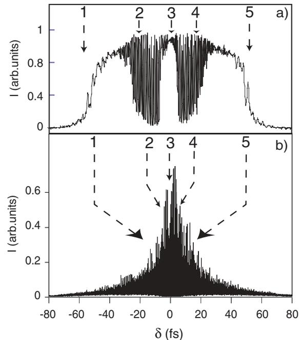
Figure 1: Detuning curve, i. e. laser intensity versus detuning obtained in the a) Super-ACO FEL, b) ELETTRA FEL. The experimental detuning curve is obtained by applying a slow ramp on the RF frequency and detecting the laser intensity by a photomultiplier or a photodiode.
