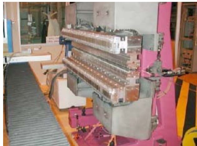
Figure 2: ESRF revolver prototype before installation in the ID18 straight section, the support is equipped with a U32 and a U20.
