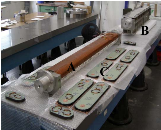
Fig. 1 The coils of the ANKA undulator before final assembly. A and B are the undulator coils during different construction phases. After coiling the wire is temporarily kept under tension in a metal container (B). After fixation the container is removed (A). C are the correction coils.
