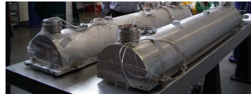
Fig. 2 Vacuum vessel (insulation vacuum) for each of the coils. The correction coils are also inside the vacuum vessel
