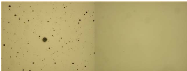
Fig. 2: Comparison between samples deposited with the unfiltered (left) and filtered (right) planar arc system. Image sizes are 252X189 \mu\text{m}
