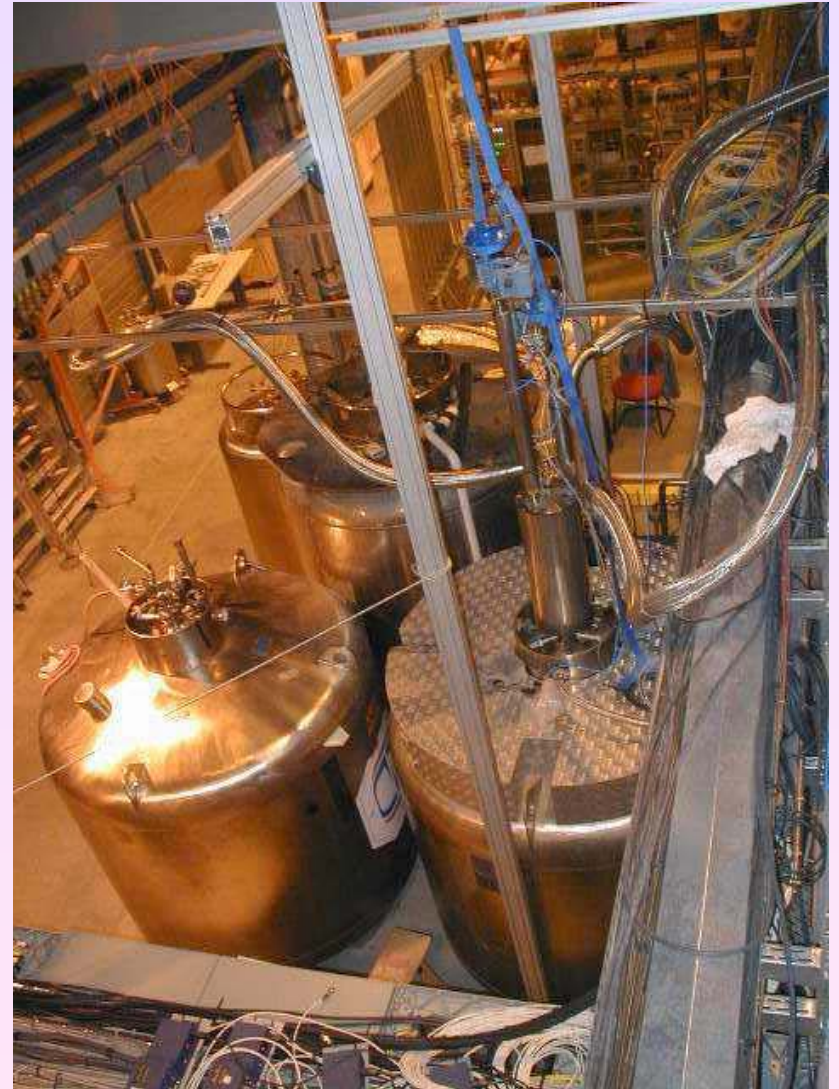
Test of SOLEIL SC Cavity Prototype on ESRF Ring, J. Jacob, slide
