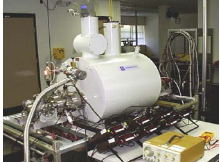
Picture of the NASA HiPAT Penning trap. This magnetic bottle was designed for the storage and transportation of 10^{12} antiprotons.
