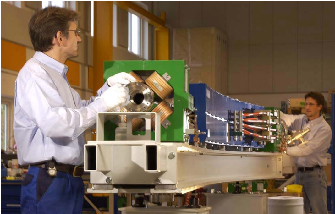
Figure 4: Pre-assembled and pre-aligned girder with one dipole magnet and two quadrupole magnets.
