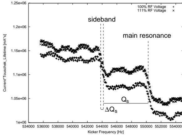
Figure 4: Dip patterns of two sweeps differing due to a 11% increase of RF voltage. The main resonance and its sideband are separated by the synchrotron tune  $Q_s = 6.17 \cdot 10^{-3}$  respectively by  $Q_s + \Delta Q_s = 6.48 \cdot 10^{-3}$  (an increase of  $Q_s$  by  $\approx 5\%$ ).
