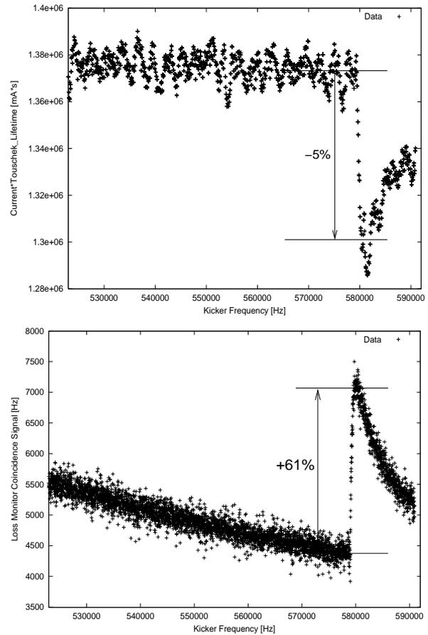
Figure 3: The resonant depolarizing frequency is reached at 580 kHz.
