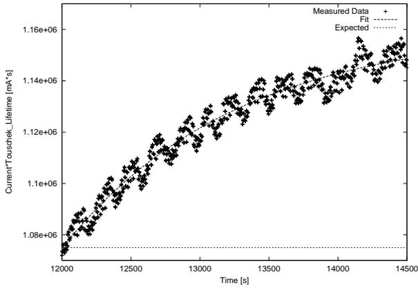
Figure 1: First observed polarization build-up and fit (flat orbit). The fit parameter for the characteristic build-up time is  $(1261 \pm 12)$  s corresponding to an equilibrium polarization of 63%. In following measurements polarization values of up to 87% were observed.
