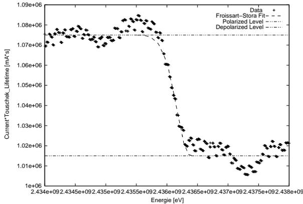
Figure 5: Resonance with fit according to the Froissart-Stora equation for resonance-crossing.
