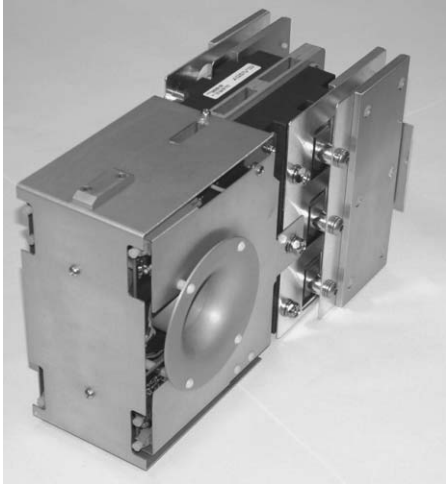
Figure 3. Dual IGBT Switch Module for the Hybrid Modulator (3.5 kV, 5000 A Peak)
