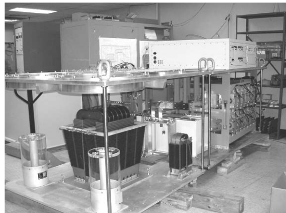
Figure 2. Hybrid modulator. Solid-state Switch (80 kV, 3500 A peak). Pulse transformer in foreground.
