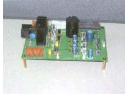
Figure 4: SRRC-2500 thyatron driver first stage circuit board
