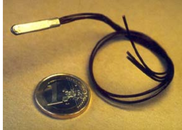
Figure 9: Connection of superconducting wires with ohmic resistance below 10^{-11} ohm
