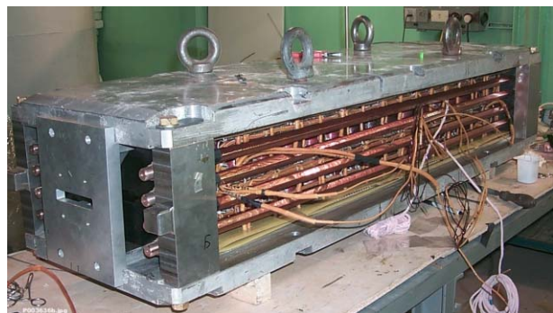
Figure 3: Wiggler magnet during assembly
