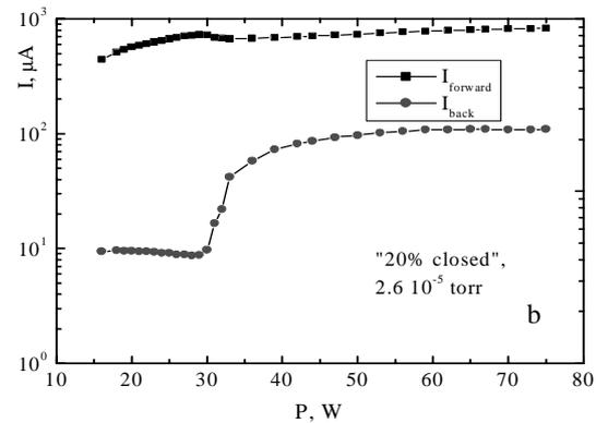
Figure 3: The variation of “forward” and “back” currents with discharge parameters: source pressure (a) and microwave power (b). 100% of holes are open.
