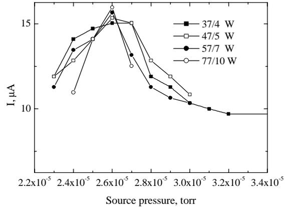
Figure 7: Measured  $Ar^{1+}$  ion current (calibrated leak 29.6  $\mu$ A) versus pressure inside the plasma chamber for different levels of direct / reflected microwave power.
