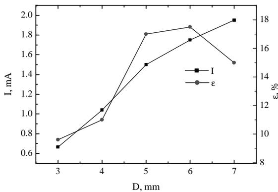
Figure 6: Maximum extracted  $He^{1+}$  current (square) and global efficiency (circle) versus the diameter of the extraction hole.
