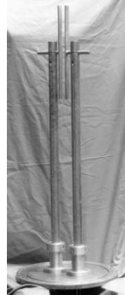
Fig. 6: Picture of the one cell funnel deflector . The deflector discs are mounted at water-cooled stems. The height is about 2 m. The cell length is \beta\lambda/2 .
