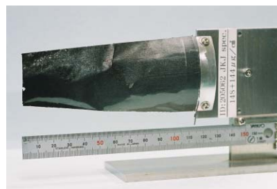
Figure 3: Overall view of the self-supported foil
