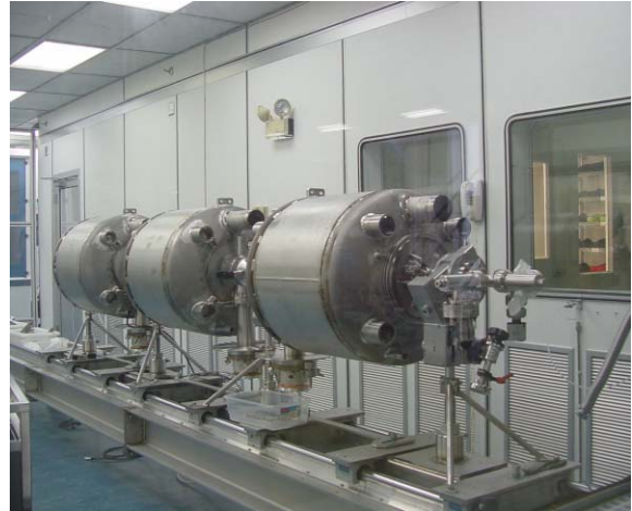
Figure 7: SNS \beta=0.61 three-cavity string assembled in the clean room.
