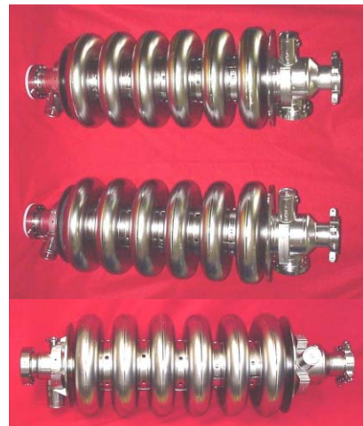
Figure 1: SNS \beta=0.61 used in the prototype cryomodule.
