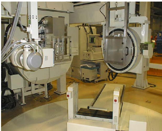
Figure 3. Patient positioning system, where treatment chair can be used with a 360 degree rotating table. There are x-ray tube (left), attachment of x-ray film with square shape and one detector (round shape) of a positron camera (right).
