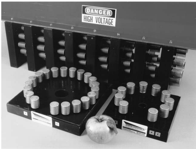
Figure 4. Solid-state switch modules and solid-state switch module assembly.
