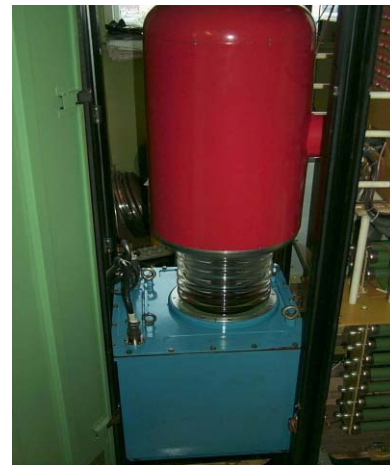
Figure 4: The picture of components of the arc discharge current source under HV potential.
