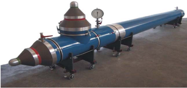
Fig. 2: 25 MVA Prototype coaxial gas insulated line KOGIL
