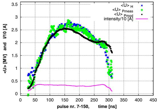
Figure 5: Energy loss estimates based on spectrometer measurements,  $\langle U \rangle_H$ , in blue (x), PETS power combined with BPM intensity measurements  $\langle U \rangle_{P_{meas}}$ , in green (o) and BPM intensity measurements alone,  $\langle U \rangle_{P_{mod}}$ , in black (+).
