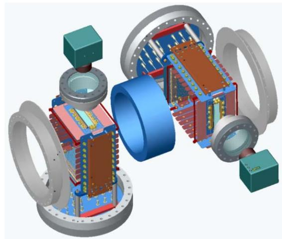
Figure 4: Horizontal and vertical IPM, separated by shielding.
