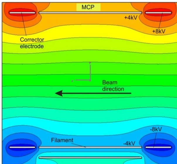
Figure 3: Longitudinal E-Field uniformity increased by corrector electrodes.
