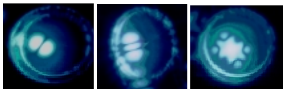
Fig. 13 : Transverse modes observed on the Super-ACO FEL, resulting from a cavity misalignment with respect to the magnetic axis of the undulator (TEM01, TEM02, TEM23).
