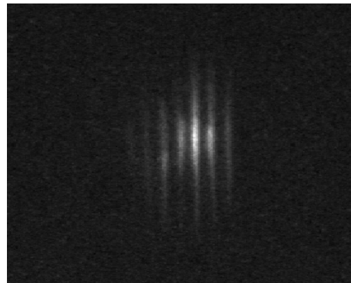
Fig. 4 – OTR image of the beam through the slits
