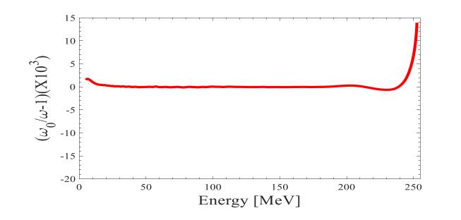
Figure 3: The isochronism parameter  $(\omega_0/\omega - 1)$  vs. energy. The  $\omega_0$  and  $\omega$  are the nominal rf angular frequency and the revolution angular frequency of particle along the SEO, respectively.
