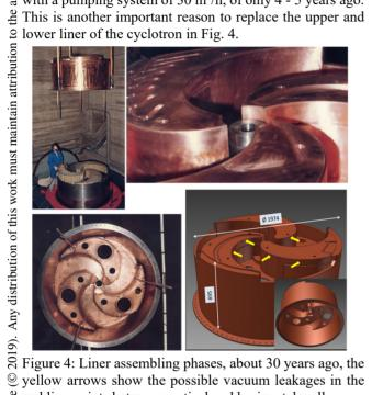
0 vellow arrows show the possible vacuum leakages in the welding points between vertical and horizontal wall.
