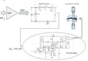
Figure 5: Block diagram of the refurbished amplifier.
