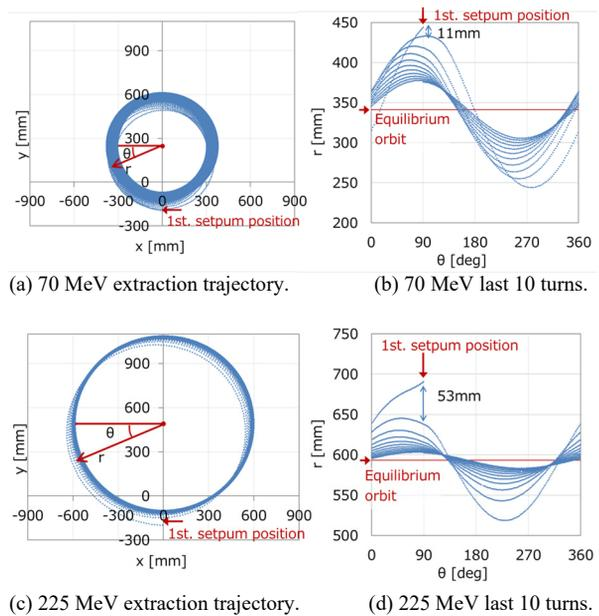
Figure 6: Tracking simulation result of beam extraction.
