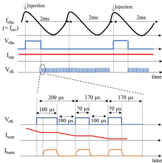
Figure 5: Timing chart of beam extraction.
