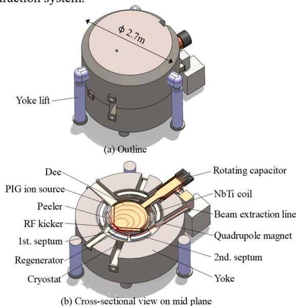
Figure 3: Schematic drawings of the accelerator.
