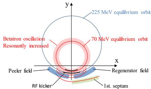
Figure 4: Schematic drawing explaining the extraction method.
