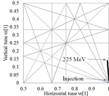
Figure 2: Tune diagram.
