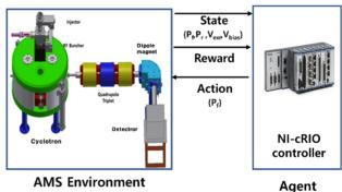
Figure 1: Reinforcement Learning based AMS control block diagram.
