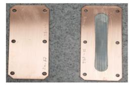
Figure 5: The copper target before and after being coated with the Zn-68.
