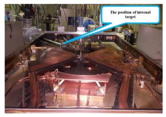
Figure 1: The normal position of the internal target during irradiation at 26.5 MeV.
