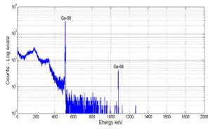
Figure 6: Characterization of Ga-68 by high purity germanium detector after production.
