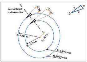
Figure 4: The target surface should be tangential to the beam orbit.
