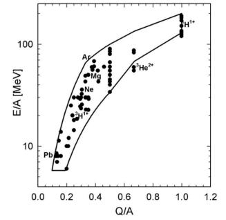
Figure 1: Operating diagram of the AGOR cyclotron.
