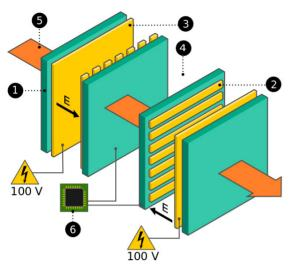
Figure 1: Schematic layout of PEPITES prototype. CP1<sup>TM</sup> membranes (1) sustain 50 nm thick gold strips (2) or are fully metallized (3). They stand in vacuum (4) where the beam (5) crosses the strips and produce secondary electrons. The signals coming from each strip are read by a dedicated readout chip (6). The final prototype will be made of 32 strips cathodes (2).
