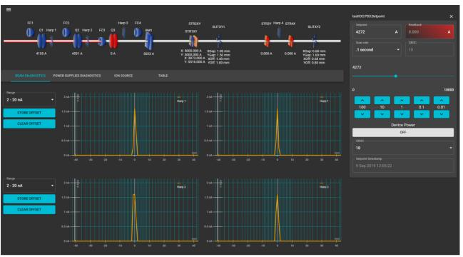
Figure 3: An example of a wide screen operator display for the control of a beam line.
