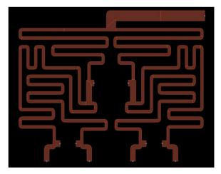
Figure 3: Pattern of the proposed 4-way power combiner circuit.
